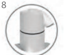
8 The 150° stop mechanism
